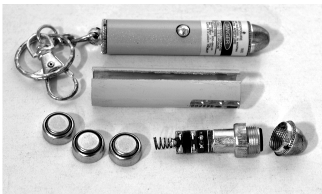
Fig. 6. The laser pointer and its constituent components. The laser diode and collimator unit is at the lower right.
