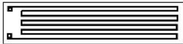
Figure 8: Strain gauge
