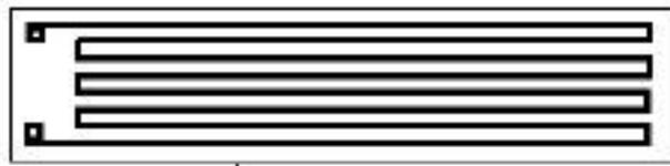
Figure 8: Strain gauge
