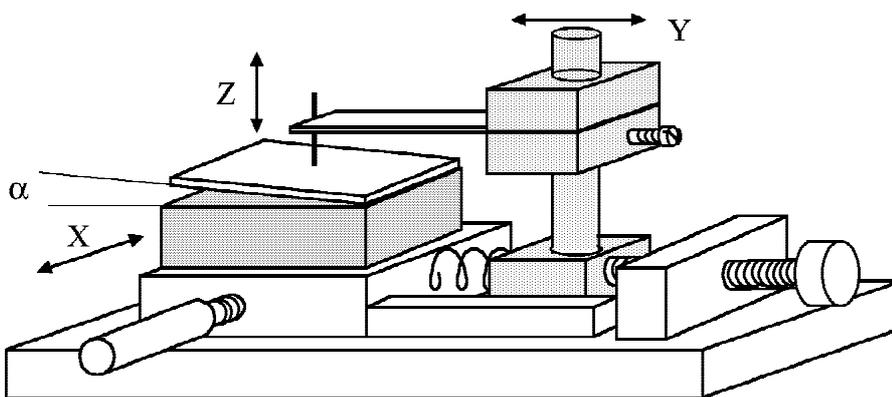
In this way each displacement  $\Delta y$  produces a fixed shift  $\Delta V_z = V(\Delta y \tan\alpha)$ , of the signal that would be measured if the sample were on the horizontal plane x,y.
