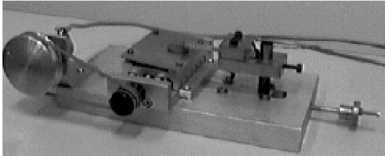
With the typical Helipot linearity (about  $10^{-4}$ ), a slide displacement of 2 mm/turn and a signal resolution of 5mV we get a theoretical resolution of  $1\mu\text{m}$ , much better than that allowed by the tip convolution and mechanical tolerances.
