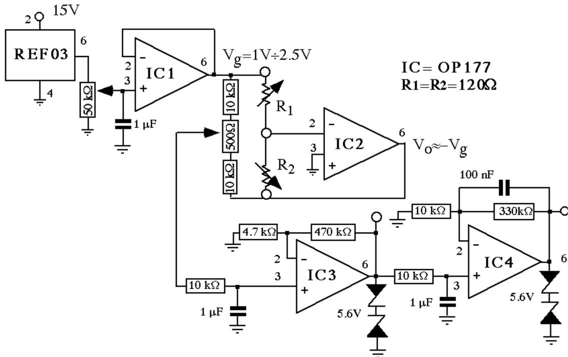
The bridge is biased at constant voltage  $V_f$  (2–5 V) through a buffer (IC1): one arm is made of the two strain gauges ( $120\Omega$ ) and the other of two fixed resistors and a balancing potentiometer.
