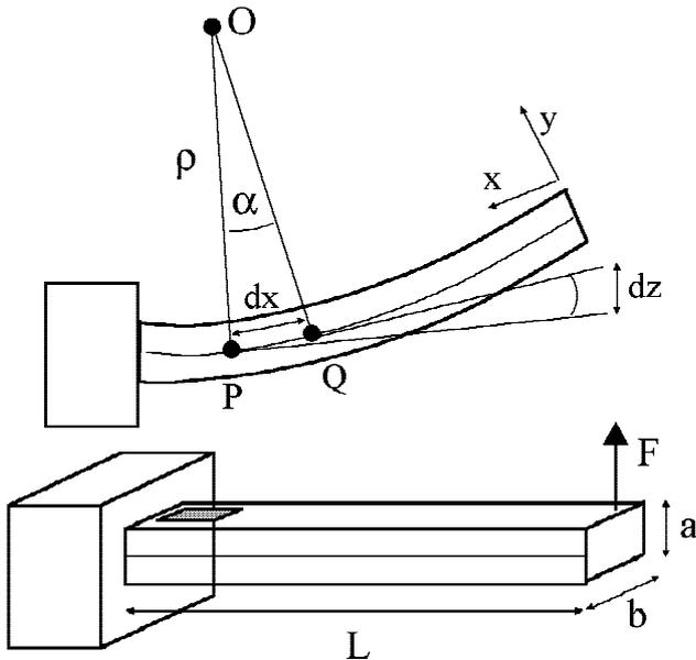
of the median fiber may be written as the product of the curvature radius  $\rho$  times the angle  $\alpha = \text{POQ}$ :  $dx = \rho \alpha$ .
