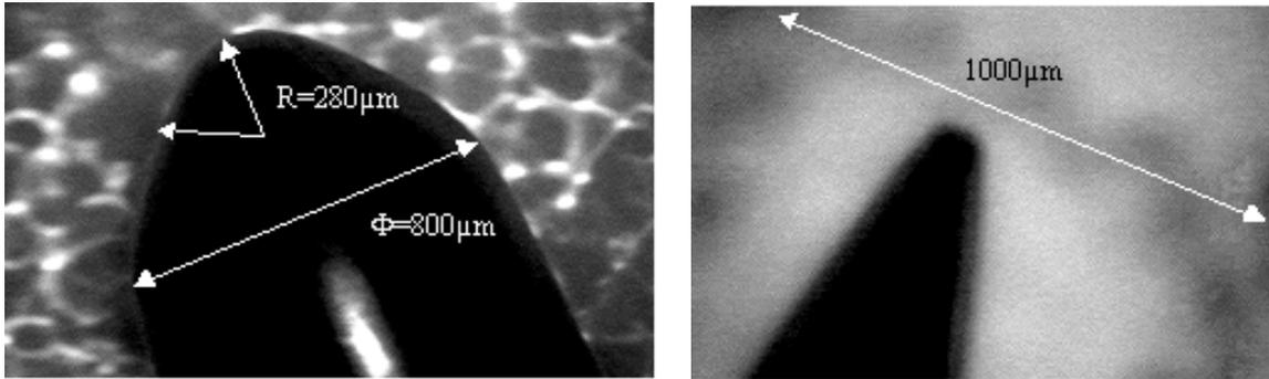
Optical micrographs of a wool-needle and of a sewing-needle tips
