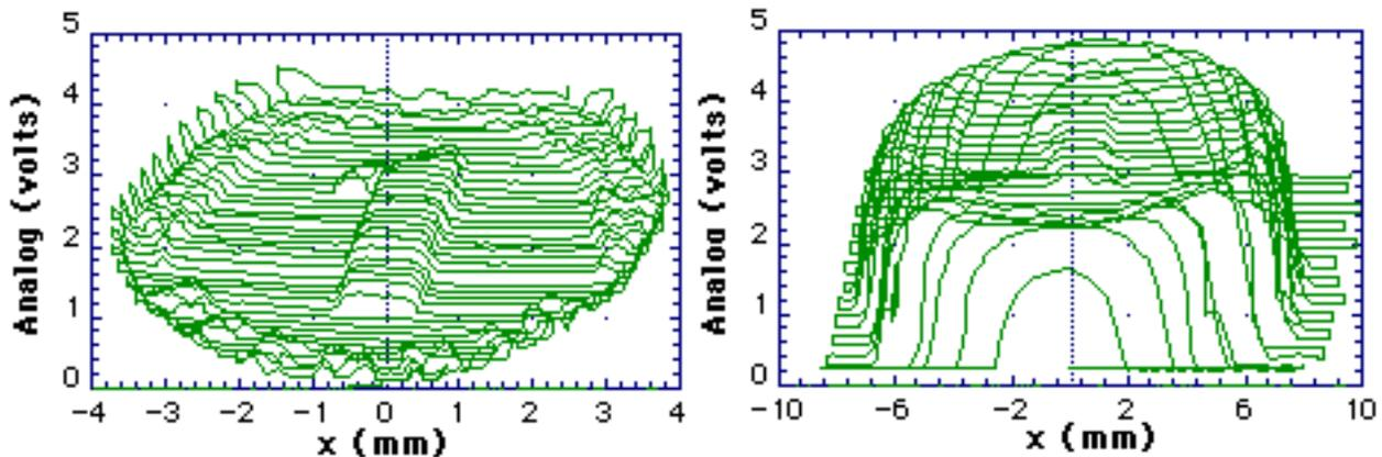
Profiles of 1 Pfennig obtained with sewing-needle and with 1.5 mm radius sphere
