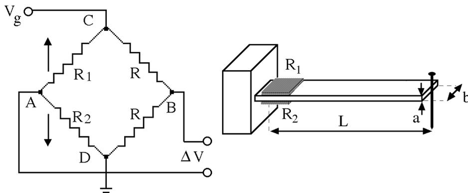
By gluing two identical strain gauges to an elastic cantilever, and by connecting them in a **Wheatstone bridge** with two fixed resistors  $R$ , we obtain a **force sensor**.
