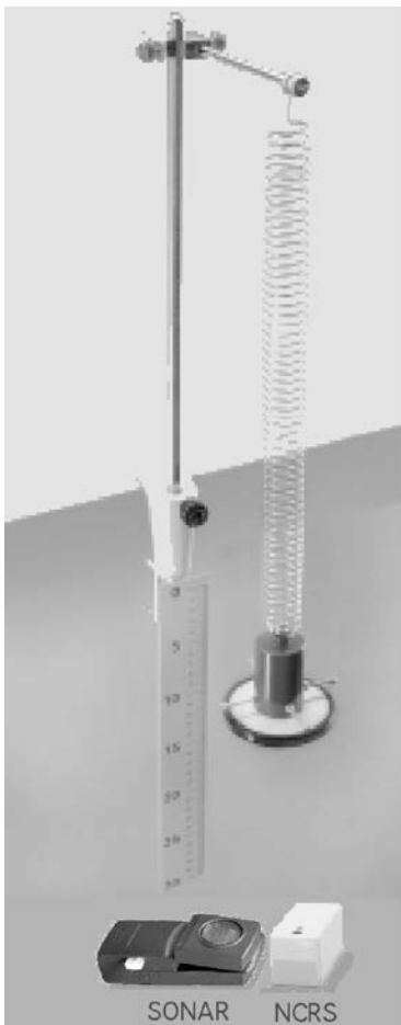
Fig. 1: The pendulum with NCRS and SONAR
